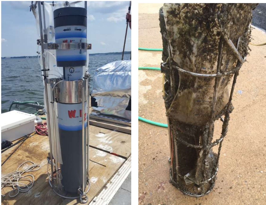
Figure 17. Photographs of the Systea-NO3 instrument prior to and following the CBL field trial.
