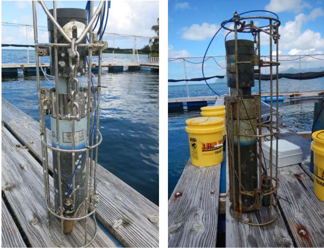
Figure 22. Photographs of the Syssta-NO3 prior to and following the one month HIMB field trial.
