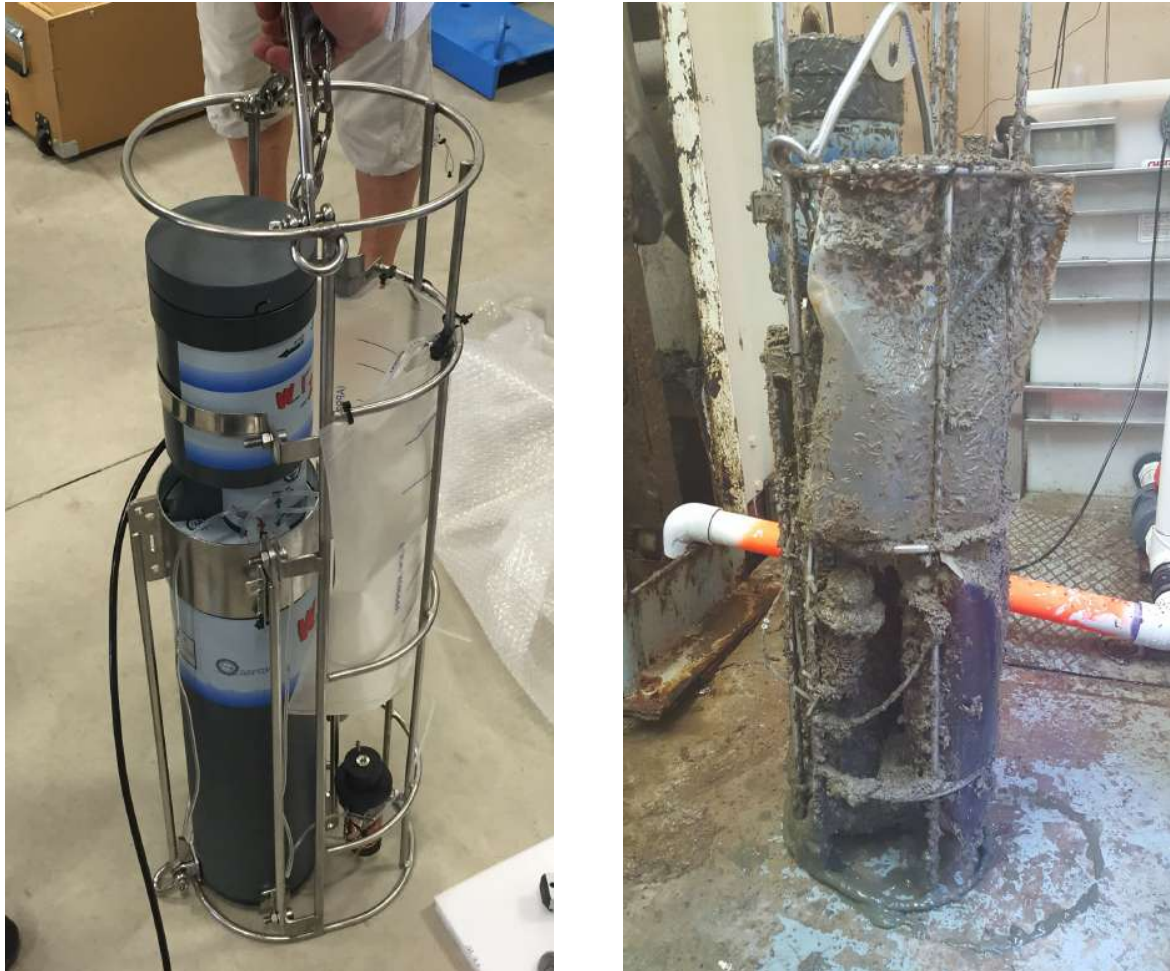
Figure 12. Photographs of the Systea-NO3 prior to and following a 32 day field test in the Maumee River.
